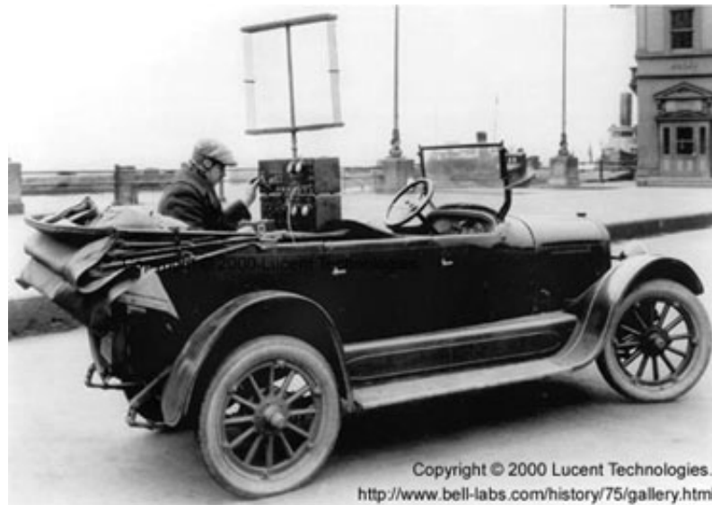
First car mounted radio telephone (1921)
