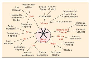
Figure: Examples of electric power infrastructure dependencies
