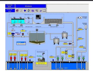
Figure: A SCADA HMI Example (fastweb.it)
