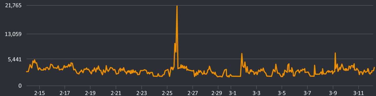
CISCO UMBRELLA SHOWING A SPIKE OF DNS REQUESTS FOR EU[.]MINERPOOL[.]PW
