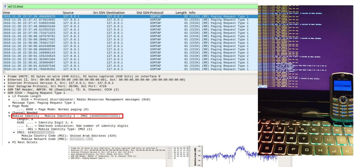
Passive IMSI Sniffing using RTL-SDR and OsmocomBB phone
