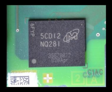
Desoldering the flash to extract firmware& application data
