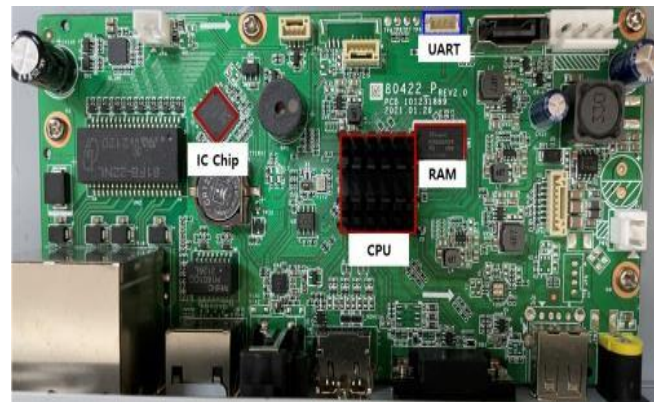
NVR equipment hardware components
