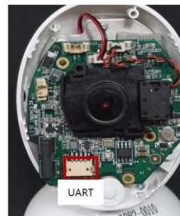
Front of IP Camera Equipment Hardware Components
